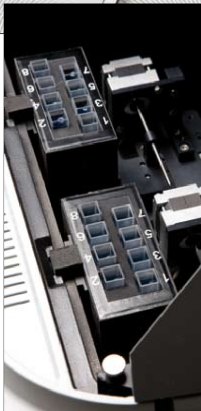
Sipper system for routine quantitative analysis
