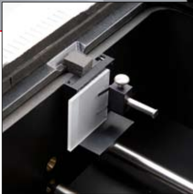
Solid sample holder to determine transmission characteristics
